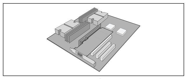
Figure 4-9. Assembled QHT7140 with Riser
